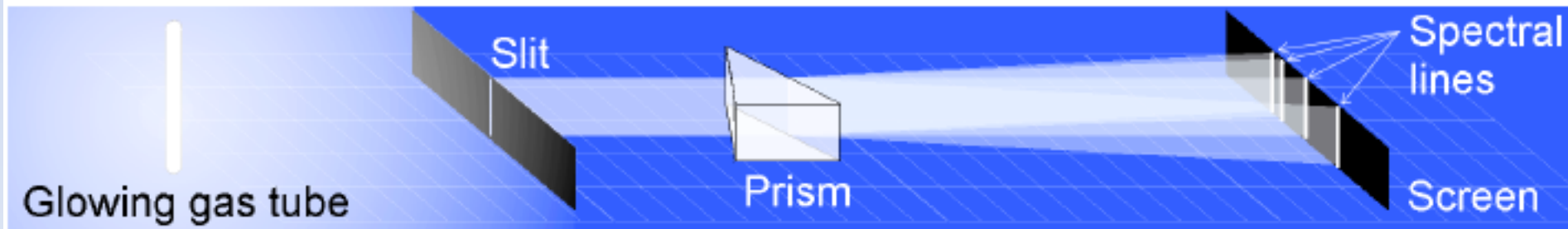
Simple prism spectrometer
